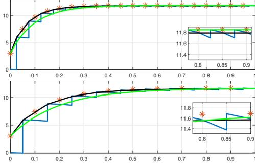
Fig. 4. Time evolution of the state variable  $x_3$  with  $p = 0.05$  s (top) and  $p = 0.1$  s (bottom): SIS (1) (blue lines), averaged model (12) (green lines), discrete-time model (16) (red stars), moving average (18) (dark lines).
