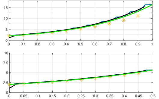
Fig. 7. Time evolution of the state variable  $x_2$  with  $p = 0.05$  s (top) and  $p = 0.1$  s (bottom): SIS (1) (blue lines), averaged model (12) (green lines), discrete-time model (16) (red stars), moving average (31) with  $\delta = p/2$  (black lines).
