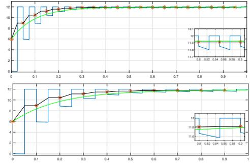
Fig. 3. Time evolution of the state variable  $x_2$  with  $p = 0.05$  s (top) and  $p = 0.1$  s (bottom): SIS (1) (blue lines), averaged model (12) (green lines), discrete-time model (16) (red stars), moving average (18) (dark lines).
