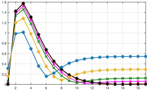
Fig. 5. Error  $\|m(t_k) - \mu(t_k)\|$  versus the multiples of  $p$  for different values of the switching period:  $p = 0.5$  s (blue line),  $p = 0.25$  s (orange line),  $p = 0.1$  s (green line),  $p = 0.05$  s (purple line),  $p = 0.01$  s (red line) and  $p = 0.005$  s (black line).
