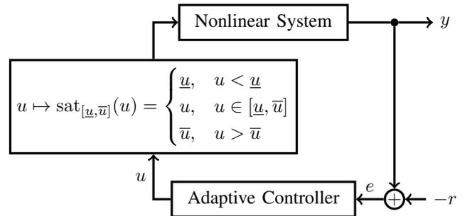
Fig. 1. Closed loop with input saturations  $\underline{u} < 0 < \bar{u}$ .
