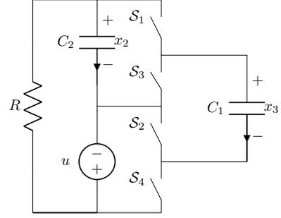
Fig. 1. Elementary cell of a ladder step-up switched capacitor converter.
