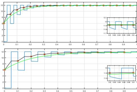
Fig. 3. Time evolution of the second state variables of the switched capacitor circuit with  $p = 0.05$  s (top) and  $p = 0.1$  s (bottom): switched DAE system (blue lines), proposed averaged model (green lines), discrete model (red stars), moving average (dark lines).
