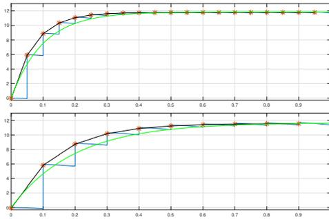
Fig. 2. Time evolution of the first state variables of the switched capacitor circuit with  $p = 0.05$  s (top) and  $p = 0.1$  s (bottom): switched DAE system (blue lines), proposed averaged model (green lines), discrete model (red stars), moving average (dark lines).
