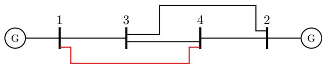
Fig. 1. A simple power grid with two generators. The red line will be subject to sudden changes in the line parameter.
