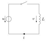
Switch  $\rightarrow$  Different DAE models (=modes) depending on time-varying position of switch
