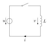
Switch → Different DAE models (=modes) depending on (time-varying) position of switch
