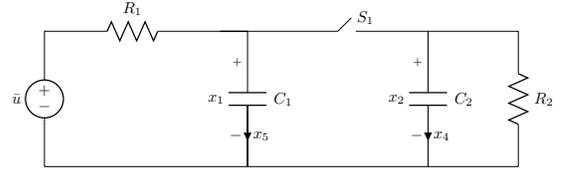
Fig. 2. A switched capacitor electrical circuit.
