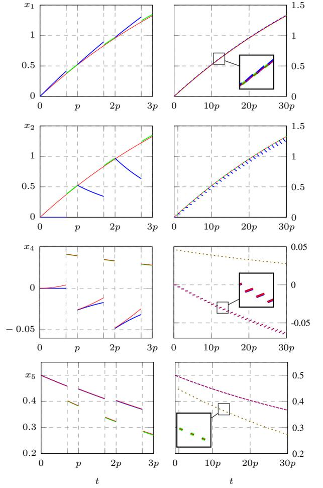
Fig. 3. Time evolutions of state components for slow switching ( $p = 0.1s$ , left) and fast switching ( $p = 0.01s$ , right). The partial averaging evolutions are plotted in red while the trajectories of the switched DAE are colored according to the active mode (mode 1 blue, mode 2 green).
