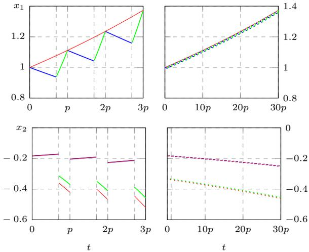
Fig. 4. Evolutions of the first two state components for slow switching ( $p = 0.1s$ , left) and fast switching ( $p = 0.01s$ , right). The averaging dynamics are plotted with red line, while the trajectories of the switched DAE are colored according to the active mode (mode 1 blue, mode 2 green).
