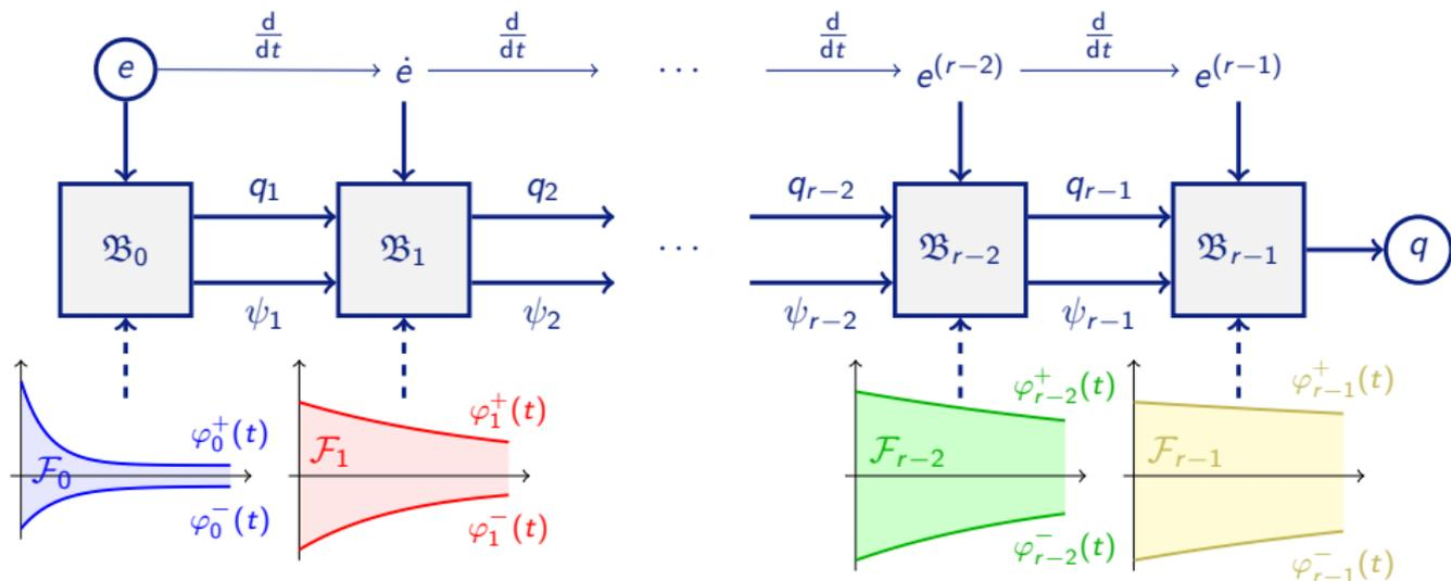
$$q_i = \text{true} \quad \Rightarrow \quad \text{Ziel: } e^{(i)}(t) < \min\{\psi_i(t), -\lambda_i^-\}$$
