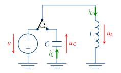
Mode 1:  $\frac{d}{dt}i_L = \frac{1}{L}u$ Mode 2:  $\frac{d}{dt}i_L = -\frac{1}{L}u_C$  $\frac{d}{dt}u_C = \frac{1}{L}i_L$
